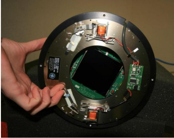
Fig. 3: MCAT’s primary detector manufactured by Spectral Instruments Inc. utilizes a 4-port 4Kx4K CCD from e2v Technologies. With 15 \mu m pixels, the focal plane plate scale is 0.75 arcsecond/pixel and the diagonal FOV is 0.96°. With 1.9-2.0 e - read noise, the detector is particularly well suited to longer exposure GEO and MEO survey work. At higher frame rates LEO altitudes to 200 km are accessible in OSM or in SCM with a high-speed shutter.
