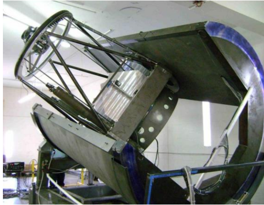
Fig. 2: A 1.3 m f/4 Ritchey Chretien telescope under construction at the DFM Engineering Incorporated facility in Longmont, CO. The OTA incorporates a 5-axis stage for secondary collimation, Invar metered truss, and a primary mirror cover. The double horseshoe mount provides a stable equatorial mount for a low latitude site with the added benefit of unobstructed north polar and south horizon access. The MCAT design is very similar to this unit.
