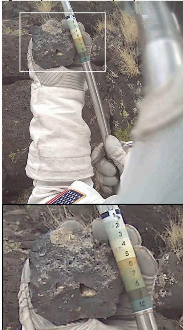
Figure 1. Image captured from suit camera video stream in real time. Crew member holds rock steady for a few seconds so that the SST can capture the image. The bottom image is an enlargement of the rock showing the detail available to characterize the sample and estimate weight.
