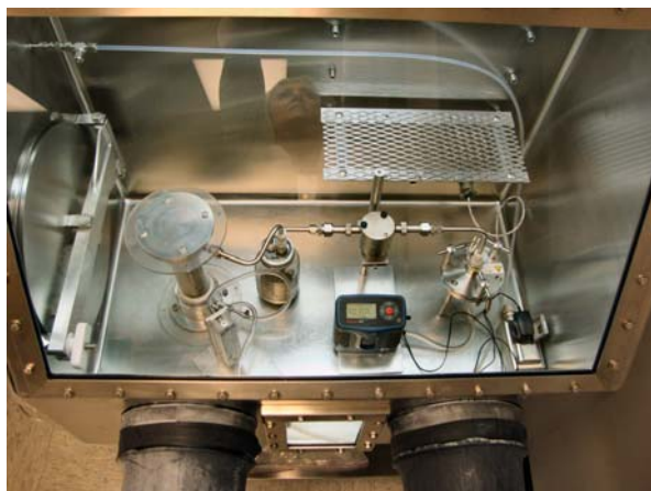
Figure 1. Dust separation system housed in a dry nitrogen glove box.
