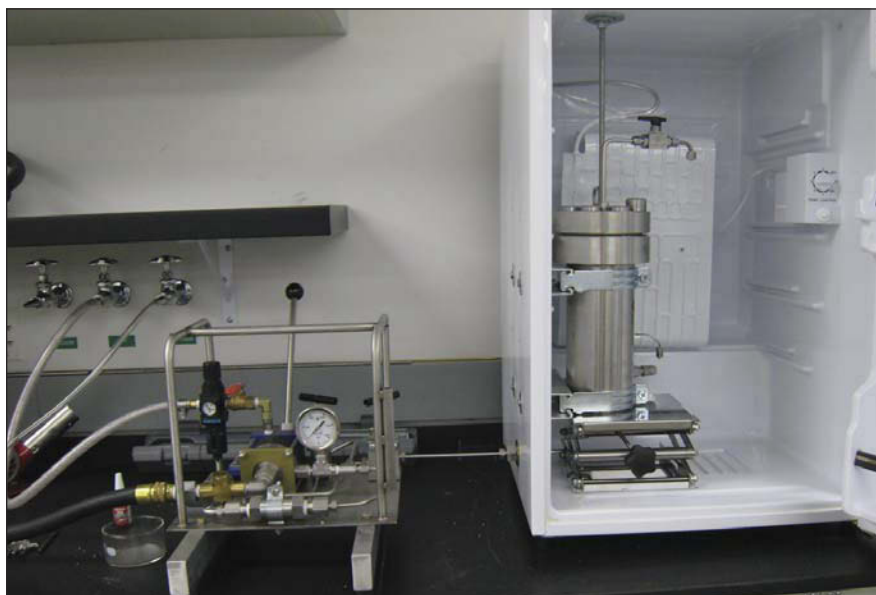
This Laboratory Apparatus is used to study biogeochemical reactions in liquid water at high pressure and low temperature. Bacterial specimens are loaded from the top of the vessel into sample cells equipped with 0.2- \mu m filters. The vessel is filled with water, air is vented from the top through a valve, and then the water is pressurized to 5 kpsi (=34 MPa).
