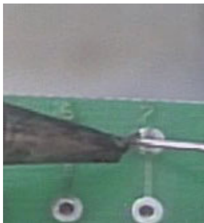
Figure 7.—Close-up image of the ISS Solder Kit soldering iron tip. The bent section of the tip is in contact with the solder wire, component lead, and circuit board plating.
