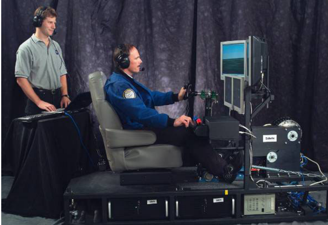
Figure 5.—NASA's Ice Contamination Effects Flight Training Device (ICEFTD).
