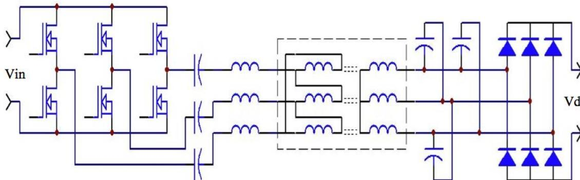
**Figure 4.** Simplified diagram of 3-phase resonant converter.
