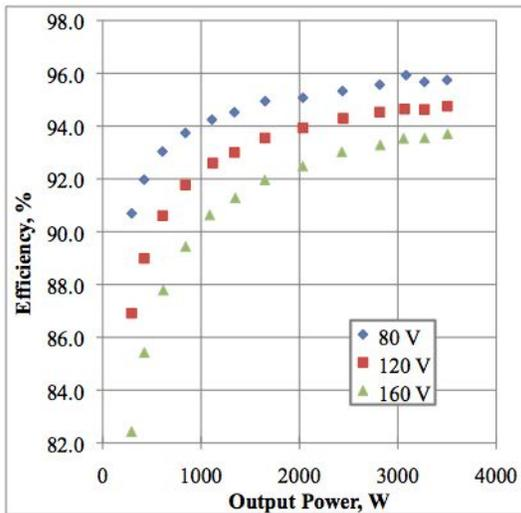
**Figure 8.** Plot of efficiency versus output power.
