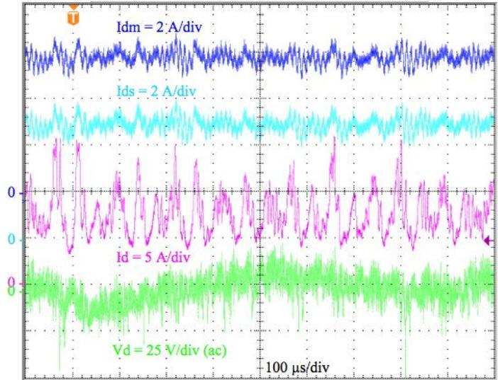
**Figure 7.** Discharge voltage and current oscillations.
