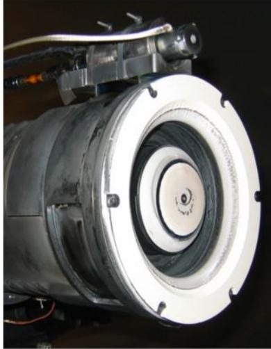
**Figure 6.** Photograph of the NASA-103M.XL thruster after 4,731 hours of testing at 700 V.
