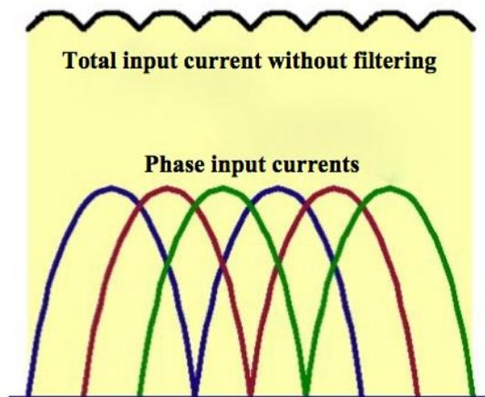
**Figure 3.** Three-phase resonant converter input currents.
