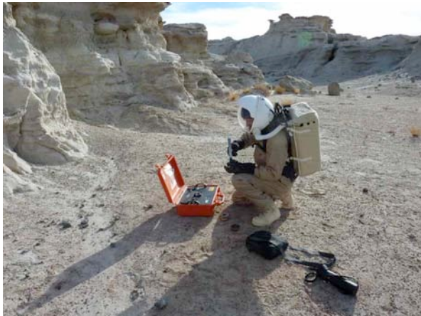
Figure 3. Terra XRD instrument operated in the field during a simulated EVA operation.
