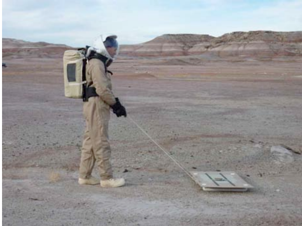
Figure 2. Collection of GPR data in the field during a simulated EVA operation.
