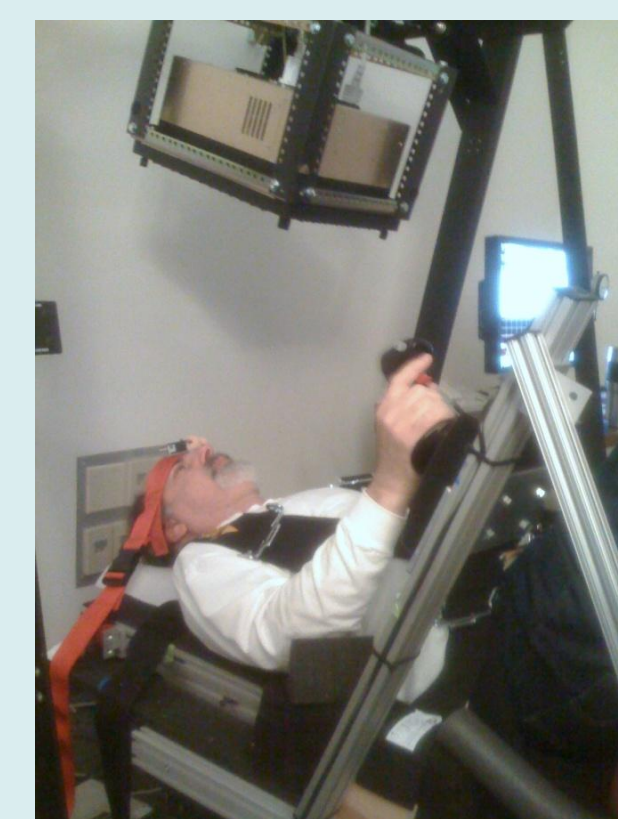
Figure 1. Semi-supine vibration seat occupant viewing display for PFD indicator assessment and post-vibration hand-flying tasks. Responses for both tasks are entered via the joystick.
