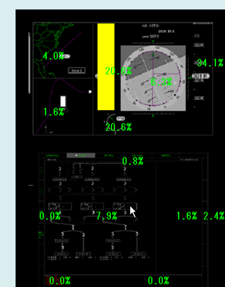
The Visualization Tool's next-fixation likelihoods, given the operator's current fixation (yellow bar) on the velocity tape of the Primary Flight Display (PFD). The operator is most likely to fixate next on the PFD's altitude tape (34.1%) or the g-meter (20.6%).
