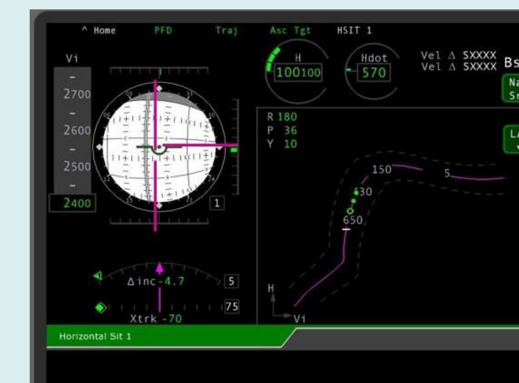
Figure 2. Rapid Prototyping Lab's prototype Orion Primary Flight Display (PFD) showing pitch rate indicator, pitch needle, and ascent trajectory predictor dots for the indicator assessment task developed in collaboration with the Astronaut Office.
