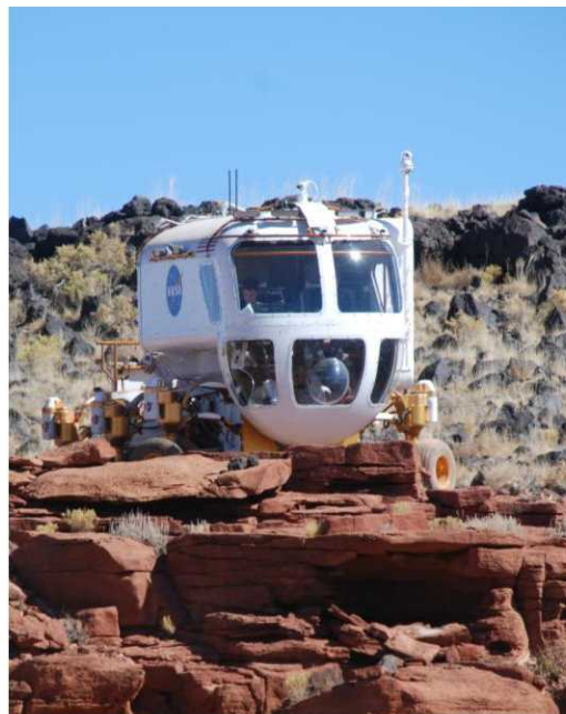
Fig.1: Prototype LER during field test at Black Point Lava Flow, in the vicinity of Flagstaff, AZ
