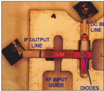
In the **Balanced Mixer**, the diodes are at the right side of the circuit and the LO comes from the waveguide at the right into a reduced-height section containing the diodes. The RF signal is picked up from the RF waveguide by the probe on the left, and flows rightward to the diodes.
