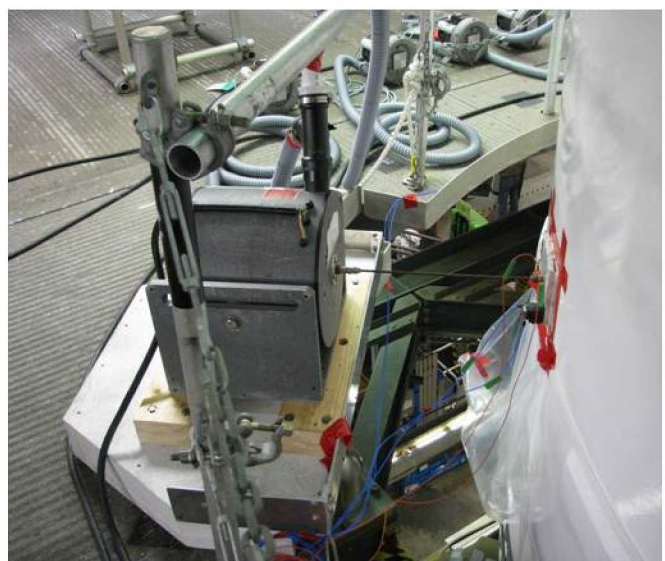
Figure 4. Electrodynamic shaker setup during Super Stack 1 modal test
