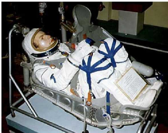
Figure D: Soyuz seat – note the higher degree of flexion in the hips and in the knees compared with the Orion seat in Figure A and B.
