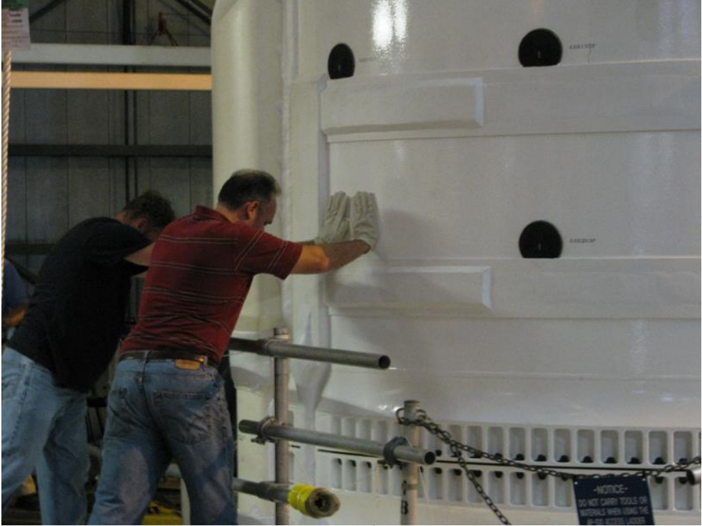
Figure 34. Manual excitation for 1 st bending mode in Y-direction.
