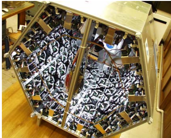
Figure 3.1: The hexagonal prism physical implementation of the test-bed, lying on its side with the end open to reveal the cellular internal structure of the electronics.
