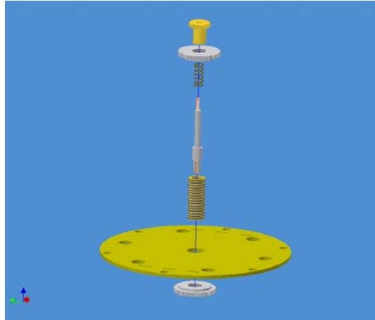
Figure 4.6: Exploded view of transducer mounted in a spring-loaded fitting that allows the position of the transducer to be adjusted relative to the CD surface.
