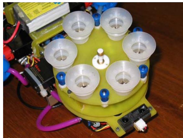
Figure 4.3: The ultrasonic transducer mounted in the centre of the robot foot.
