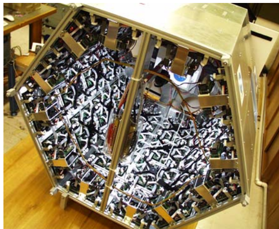
Figure 2.1: The hexagonal prism physical implementation of the test-bed, lying on its side with the end open to reveal the cellular internal structure of the electronics.
