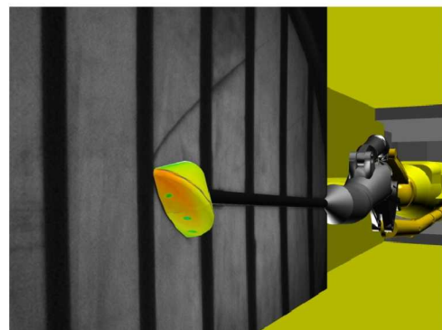
Figure 12. Post-test data visualization showing IR camera thermal imagery mapped onto the Orion capsule with corresponding Schlieren flow visualization imagery.
