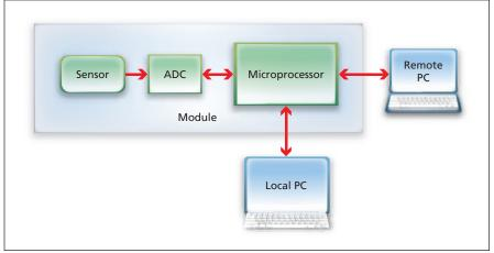
The **"Smart" Sensor Module** is programmed by use of the local PC and thereafter operated by the remote PC. In addition to preprocessed sensory data, the module generates an indication of the reliability of the data (and, hence, of the health of the sensor).
