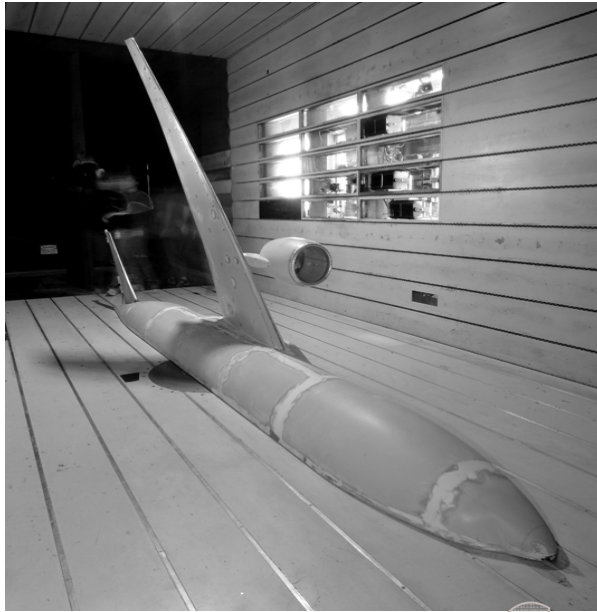
Fig. 2 a) A typical Boeing semi-span model installation in the 11-By 11-Ft TWT at the NASA Ames Research Center and b) a semi-span model sealed to the floor with aluminum high speed tape.
