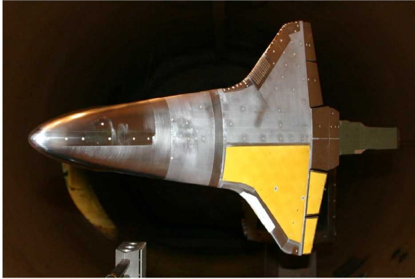
Figure 23. MH-13 Model Overview Showing Yellow Temperature Sensitive Paint Regions
