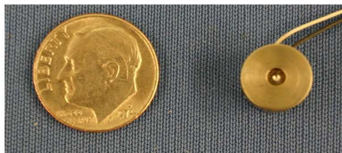
Figure 9. Typical PCB Piezoelectric Pressure Transducer
