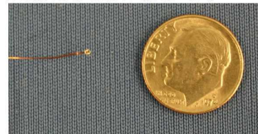
Figure 6b. 0.050" Thin-film Heat Transfer Instrument
