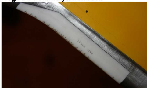
Figure 8. Macor Insert in Starboard Wing Leading Edge
