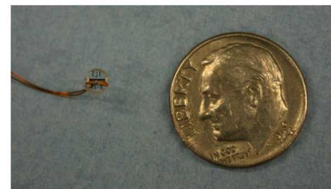
Figure 6b. 0.125" Thin-film Heat Transfer Instrument
