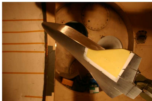
Figure 19. Aluminum Temperature Sensitive Paint Risk Mitigation Model
