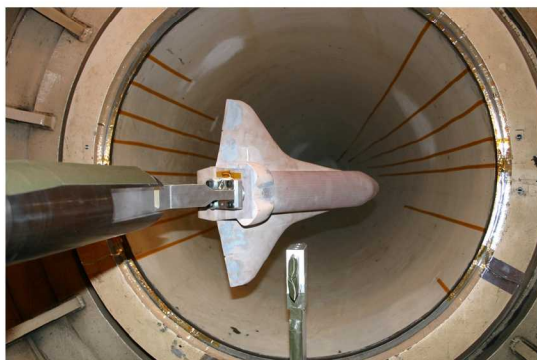
Figure 18. RenBoard Temperature Sensitive Paint Risk Mitigation Model
