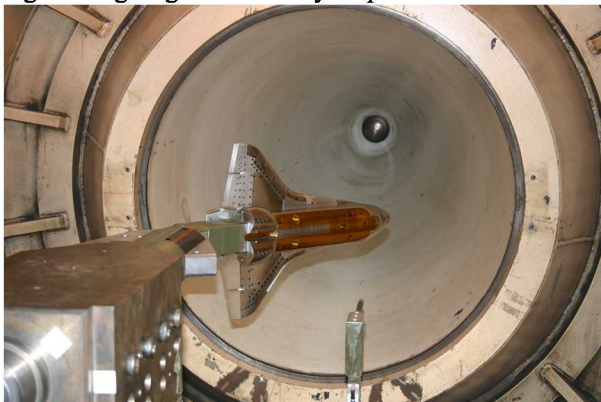
Figure 21. MH-13 Aerothermal Model Installed in LENS I
