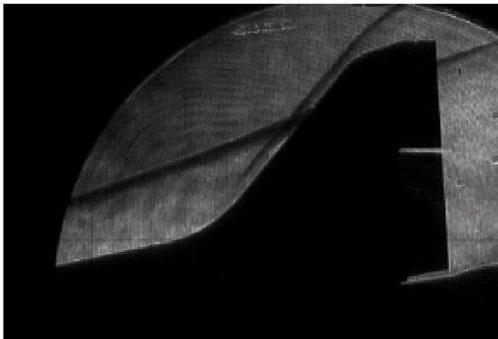
Figure 16. Typical Schlieren Image of Shock Interaction Due to Bow Shock from Orbiter Nose
