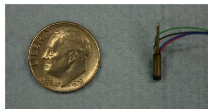
Figure 10. Typical Kulite Piezoresistive Transducer
