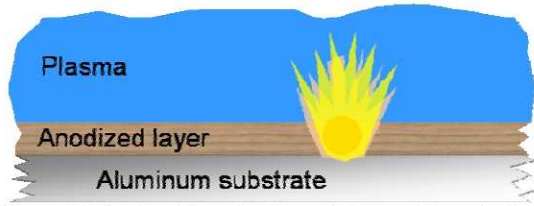
Figure 7. Arcing. Electrical breakdown of chemical coating on aluminium structural elements.
