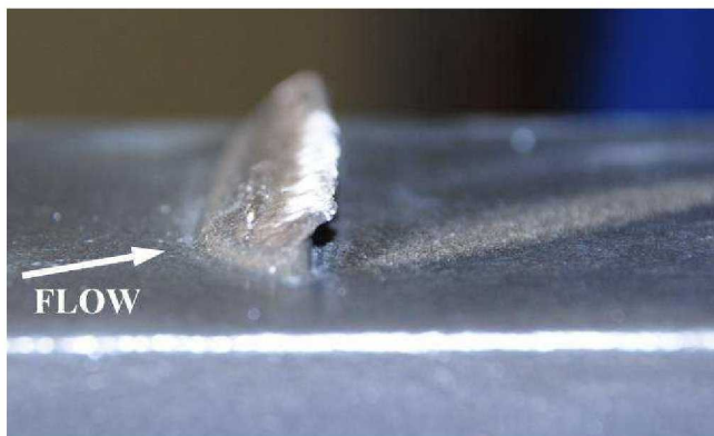
Figure 10. Post-test photograph of the slumped protuberance trip.
