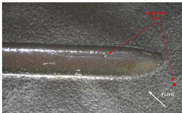
Figure 7. Post-test photograph of the 0.35-inch protuberance showing RCG coating discoloration and partially exposed thermocouple bead.
