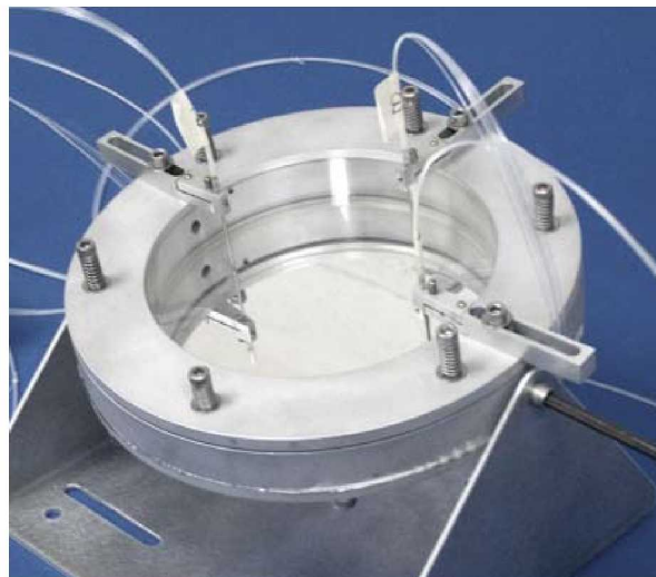
Figure 1. Rear view of a typical FOMIS test system with three FOD sensors mounted on support arms
