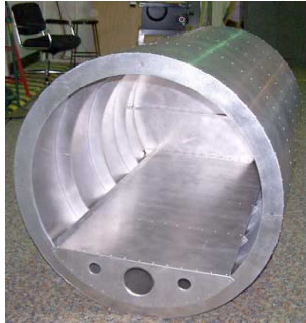
Figure 3. Scale model of a lunar habitat instrumented with 20 PINDROP sensors.
