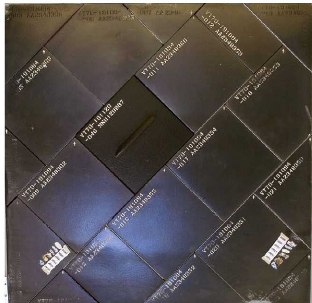
Figure 1. Pre-test photograph of the variable configuration tile array with protrusion tile insert ( k = 0.35 in.)
