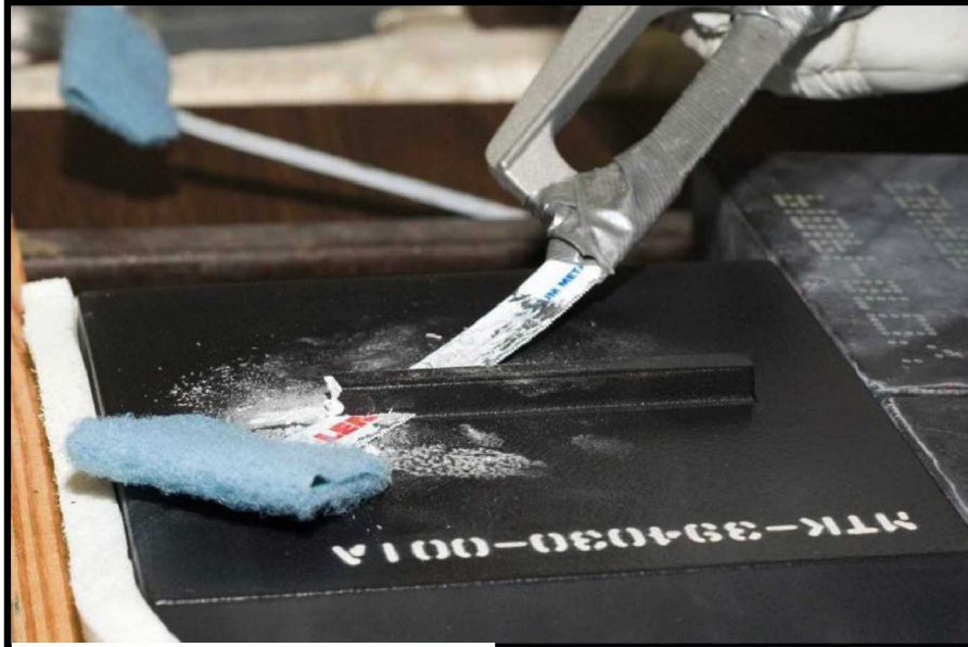
Figure 2. Tile protuberance prototype being cut by an EVA hacksaw (Ref. XX)
