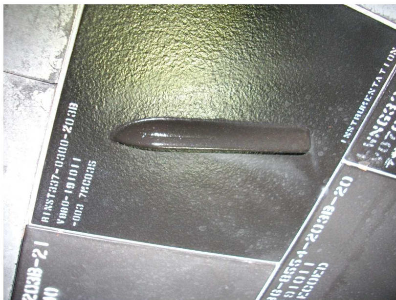
Figure 18. Post-flight runway photograph of STS-128 (0.35-inch) protuberance.
