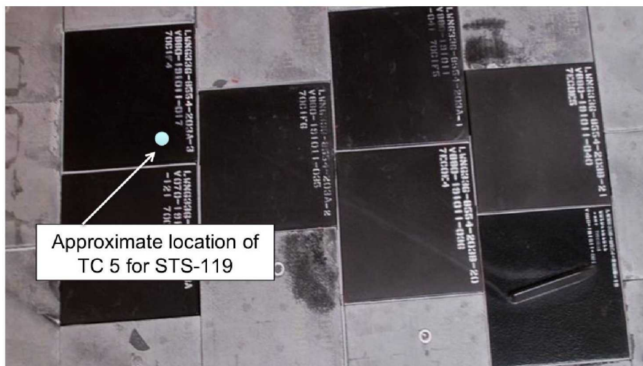
Figure 11. STS-119 post-flight photo showing streamline structure
