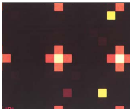
This Difference Image from a portion of an image detector containing a rectangular pixel array was generated from two images: one recorded immediately after and one recorded immediately before the second reset. The second-reset pixels were those residing at intersections of rows and columns at seven-pixel intervals.
