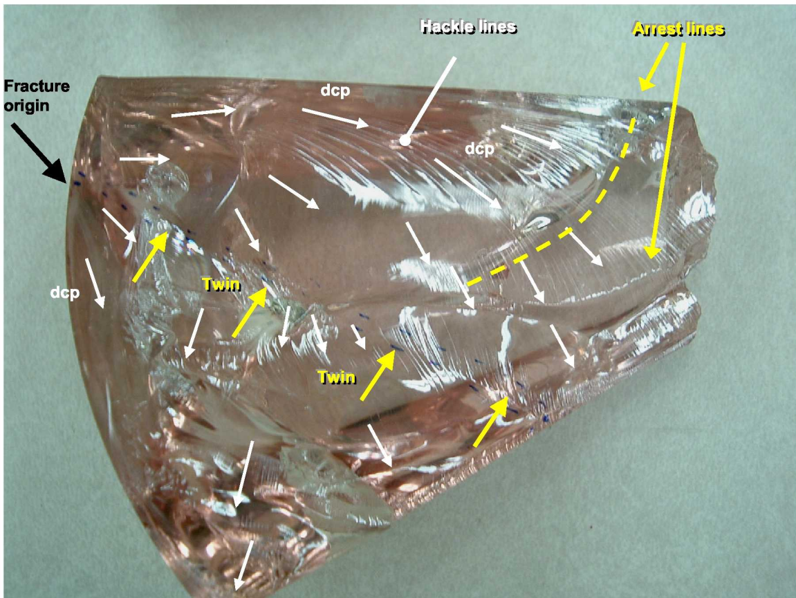
Figure 8.—Piece 2 of RSC no. 1. The small white arrows show the local direction of crack propagation (dcp) as identified by hackle lines, Wallner lines (not labeled), and arrest lines. These facilitate the determination of the crack propagation direction and the fracture origin. The twin runs diagonally across this view as marked by yellow arrows. Its left end comes very close to but is not coincident with the fracture origin. The main crack was perturbed slightly when it traversed across the preexisting twin.
