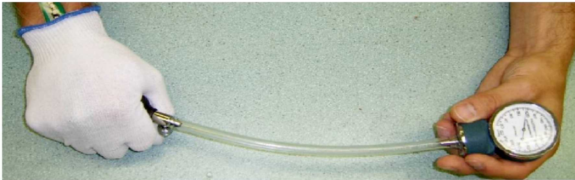
Figure 7.—A subject demonstrating use of the sphygmomanometer assembly during testing. The pressure exerted by the bulb represents the force from gripping an EVA tool.
