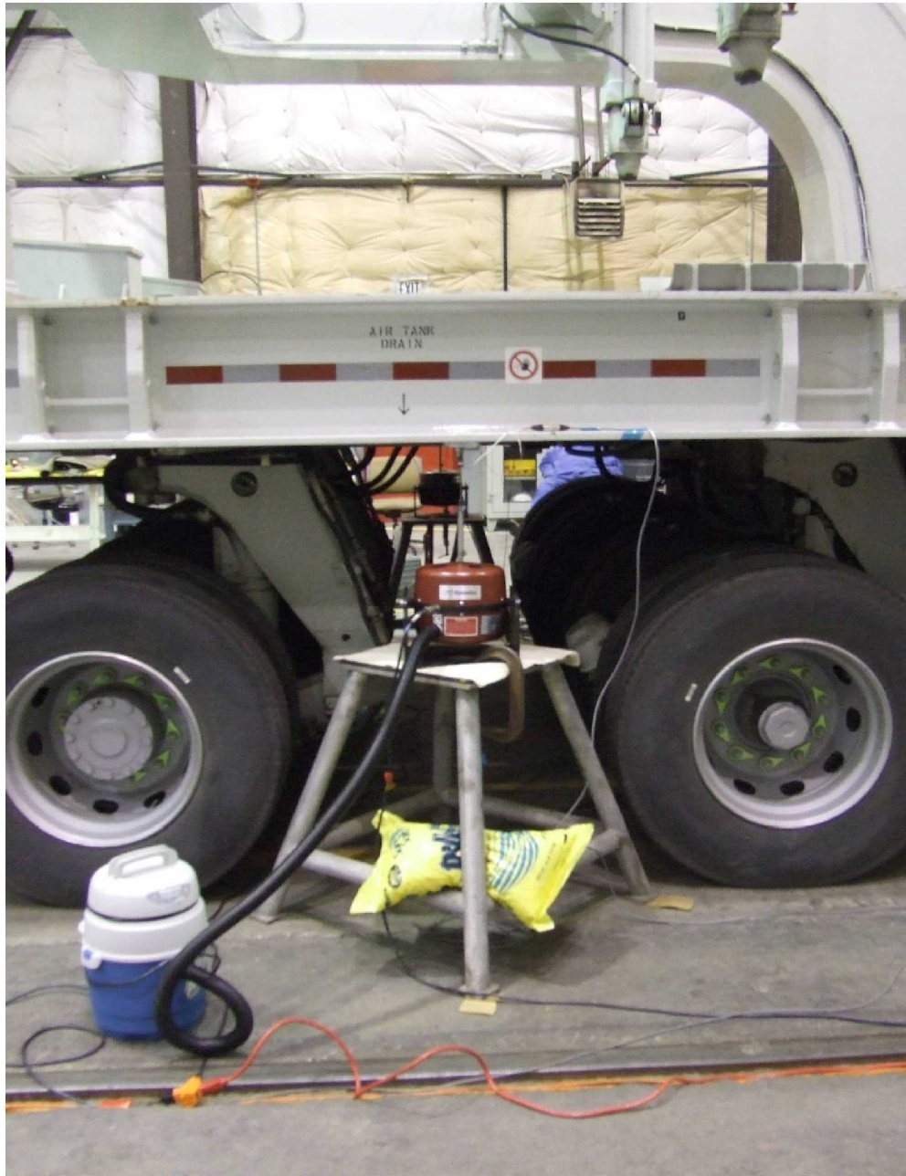
Figure 5. Shakers were installed atop stands under the trailer frame.
