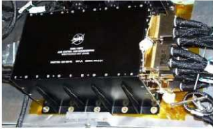
ASTRO-E2 XRS Detector with Cryo Cables, and ADR Control Electronics
