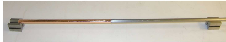
11) Evaporator covered with copper leaf, 1.27 cm O.D., full length view, #11
