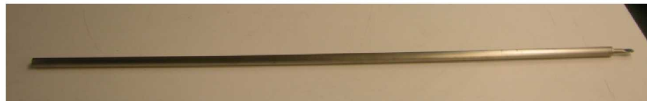
10) Plain Evaporator, 1.27 cm O.D., full length view, #10.
