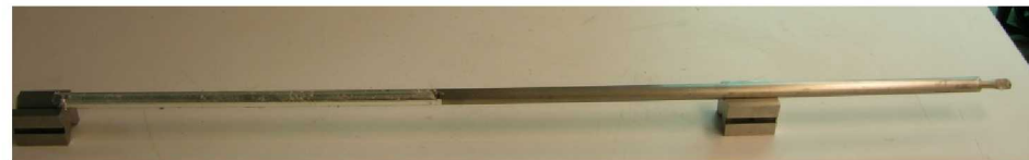
12) Evaporator covered with silver leaf, 1.27 cm O.D., full length view, #12
