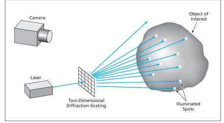
A **Diffraction Grating Would Split a Laser Beam** into multiple beams to project a grid of bright spots onto an object of interest. A camera offset from the laser and diffraction grating would capture an image of the illuminated spots. The 3D positions of the spots would be computed from their positions in the image by triangulation.
