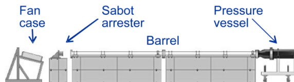
Figure 14.—Schematic of the gas gun and the fan case mounted at an incline in front of the gun barrel.
