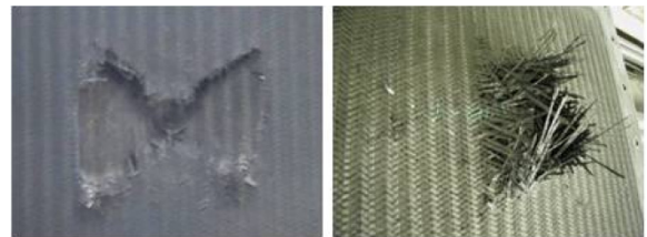
Figure 13.—Failure modes observed for different material systems showing crack propagation along bias fiber directions (left) and fiber brooming (right).
