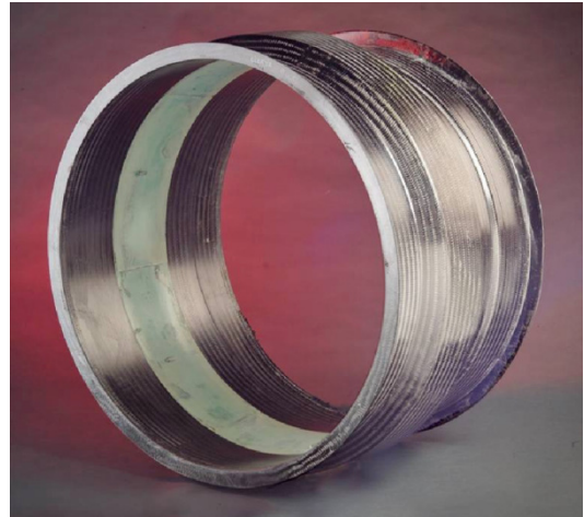
Figure 2.—Composite softwall fan case prototype.
