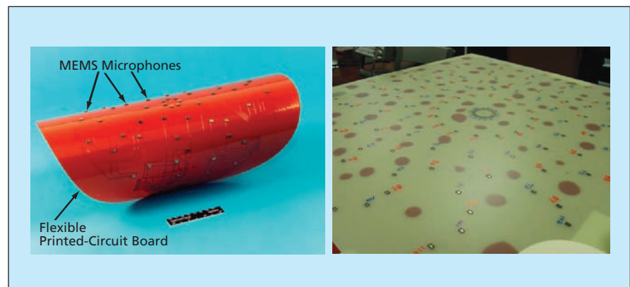
An Array of MEMS Microphones (left) and a Face Sheet (right) are shown. The array is formed on a flexible printed-circuit board. The array can readily be affixed to a curved wind-tunnel surface for use in aeroacoustic testing. The face sheet containing small rectangular cutouts for the microphones is placed over an array like that on the left to provide a smooth outer surface.
