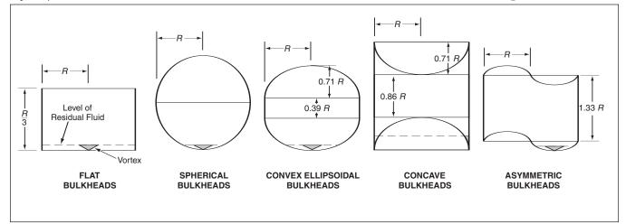
These **Pressure-Vessel Configurations** have the same radius (*R*) and volume ( $4\pi R^3/3$ ). The different shapes are shown here to illustrate the advantages and disadvantages of each. This is a representative but not exhaustive set of configurations, and is limited to single, non-nested pressure vessels for the sake of simplicity.
