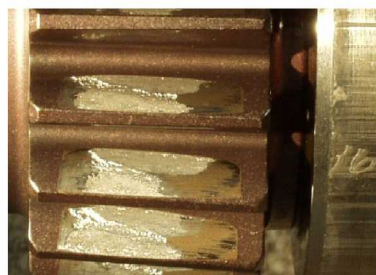
(b) Multiple teeth macro-pitting failure.
