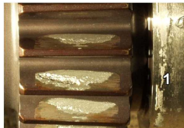
(a) Single/few teeth macro-pitting failure.
