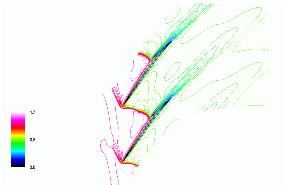
Figure 7(c).—Mach number distribution at 70% span, near peak efficiency, rotor design speed.
