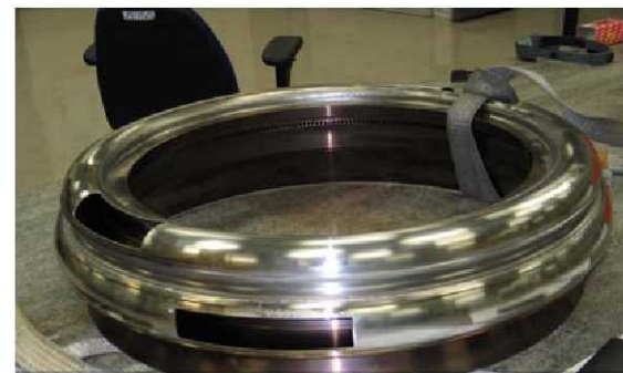
Regen Nozzle Forward Manifold Weld MTD in PMR for Inspection
