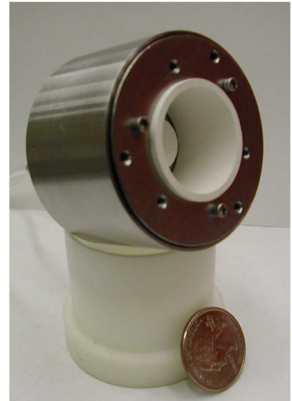
Figure 2. Laboratory model 2.6 cm CHT with Sm-Co permanent magnets (with US quarter for scale).
