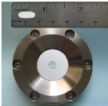
Figure 2. Coaxial GEM thruster electrodes, and boron nitride insulator.
