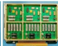
Built Up Initiator Firing Circuit (IFC) Module PWB - ISC/RCU
