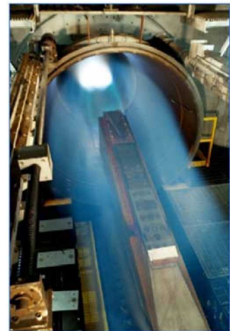
Figure 1. The X51-A hardware (SjX61-2) installed in the NASA LaRC 8'HTT Facility.
