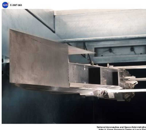
Figure 5.(a) The IMX model Mach-4 configuration installed in the NASA-GRC 1’x1’ SWT Facility.
