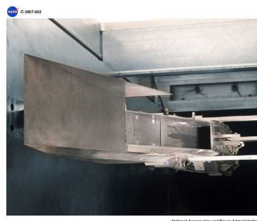
Figure 5. (b) The IMX model Mach-7 configuration installed in the NASA-GRC 1’x1’ SWT Facility.
