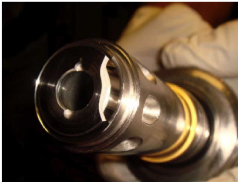
Figure 2. Poppet head breakage of gaseous H_2 flow control valve on STS-126.
