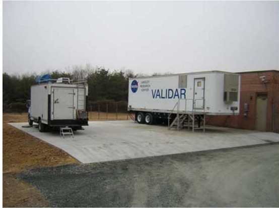
Figure 1: Photograph of field test site at the Howard University Research Campus in Beltsville, MD. The lidar is housed within a 35-foot long trailer testbed called VALIDAR. The other trailer houses the Goddard Lidar Observatory for Wind (GLOW).
