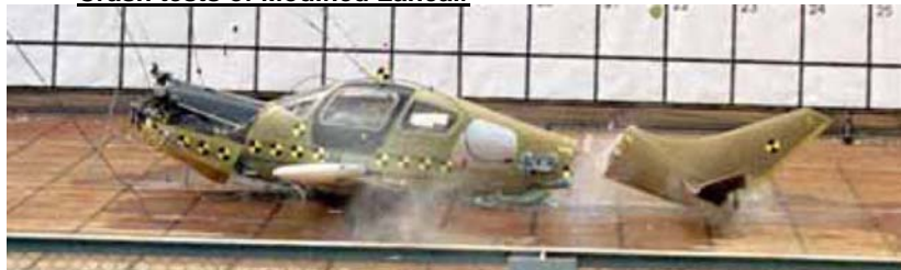
Crash tests of Modified Lancair
