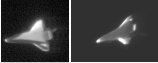
Figure 11. Unprocessed infrared images of STS-119 (left) and STS-125 (right).
