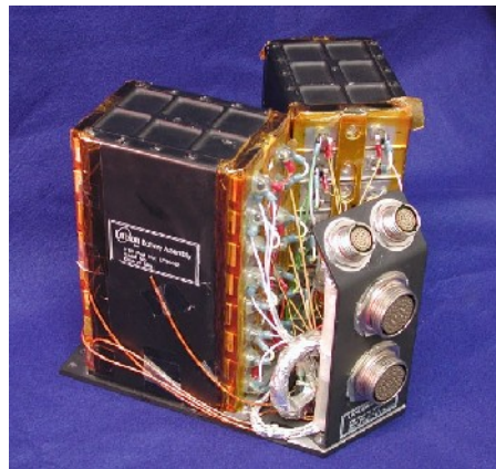
Figure 5.12—Example Li-Ion Battery, Built for the Mars Phoenix Lander (Similar Batteries are Planned for Orion)
