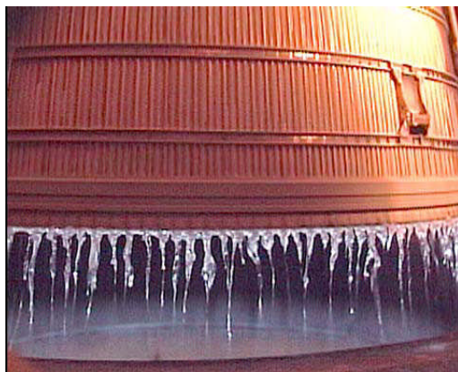
Figure 7. CECE at 30% Power Levels Showing Ice Formation
