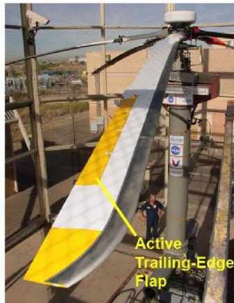
Figure 3. Boeing-SMART rotor with active trailing-edge flap.
