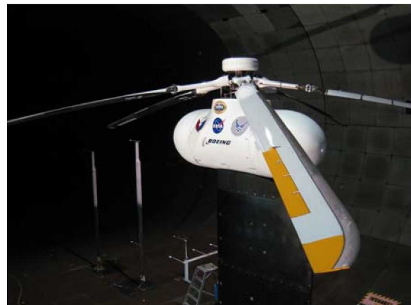
Figure 2: Close-up view of the SMART rotor, blade, and flap
