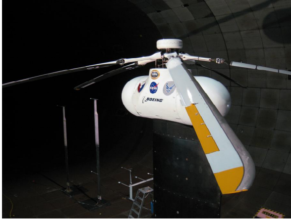
Figure 3b: Close-up view of the SMART rotor, blade, and flap in the tunnel
