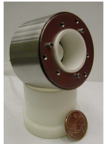
Figure 1. Laboratory model 2.6 cm CHT with Sm-Co permanent magnets (with US quarter for scale).
